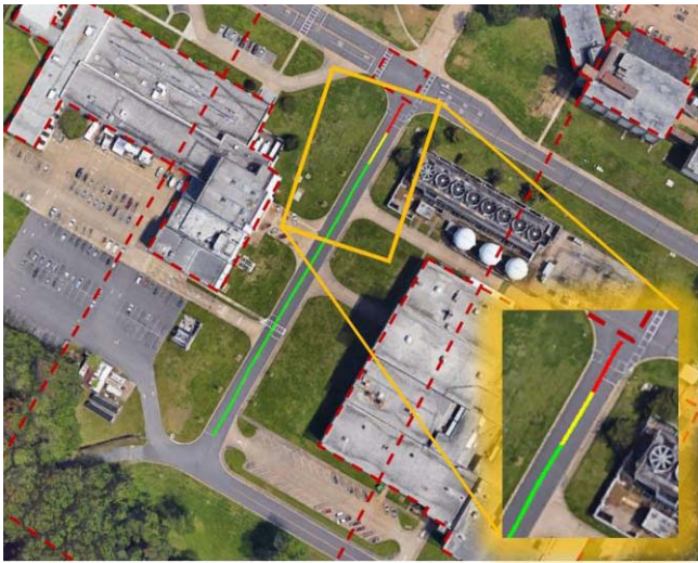
Figure 9. Flight Results from Operational Scenario 2 with Simulated Autopilot Failure and Terminate Signal Triggering Land Maneuver.
