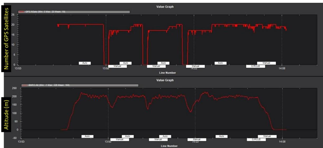
**Figure 9. GPS Failure Effect on Altitude.**
