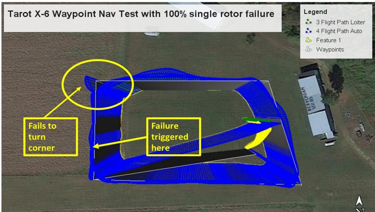
Figure 6. Tarot X6 Waypoint Navigation with Rotor Failure.
